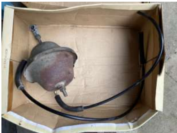
the double acting servo for the pop up head lamp pods and some pipe work
